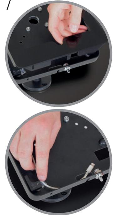
Lift fascia out of enclosure. Gently press cable (supplied with Apple iPad) into retaining moulding, allowing 10cm to remain "free" at charge/sync connector end.
