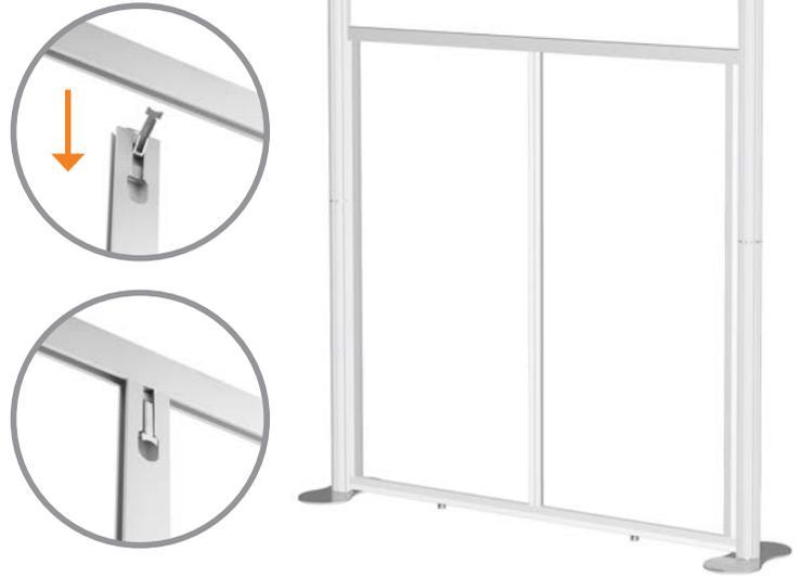
Connect second 1500mm horizontal (H) using the T-Loc clamps, to top of assembled verticals (V, V and V1) Close T-Loc levers on vertical rails to secure, then close T-Loc levers on horizontal (H)
