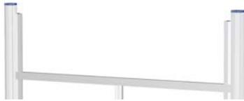
Ensuring the single steel strip of 355 vertical (V2) rail is adjacent to post, slot T-Loc clamp into channel of horizontal (H) at corner. Close bottom T-Loc lever to secure and repeat for opposite vertical rail.
