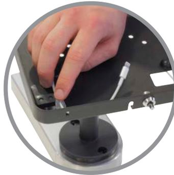
Lift fascia out of enclosures. Insert cables (supplied with Apple iPad) into both holders, allowing 10cm to remain "free" at charge/sync connector end by gently pressing into retaining moulding.
